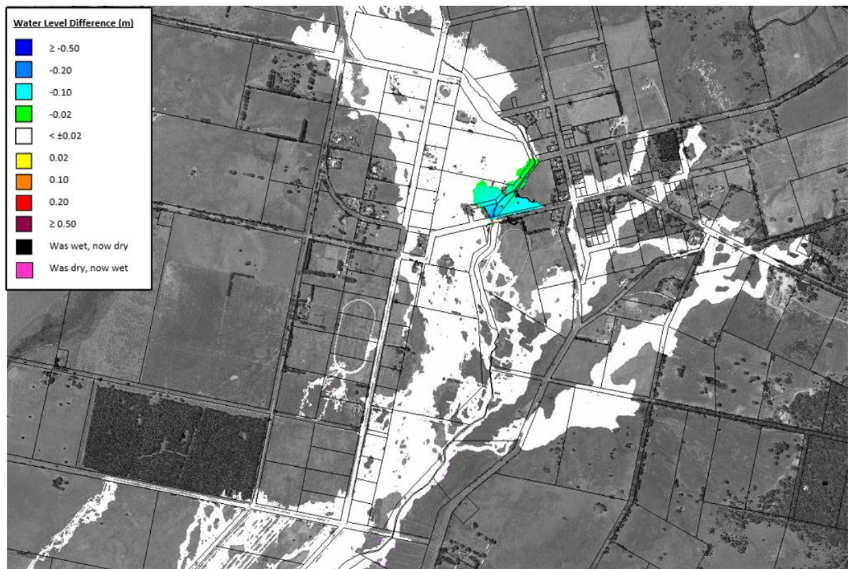
Plate 8 - 1% AEP change in flood levels due to widening the Fiery Creek crossing at Raglan - Elmhurst Road
