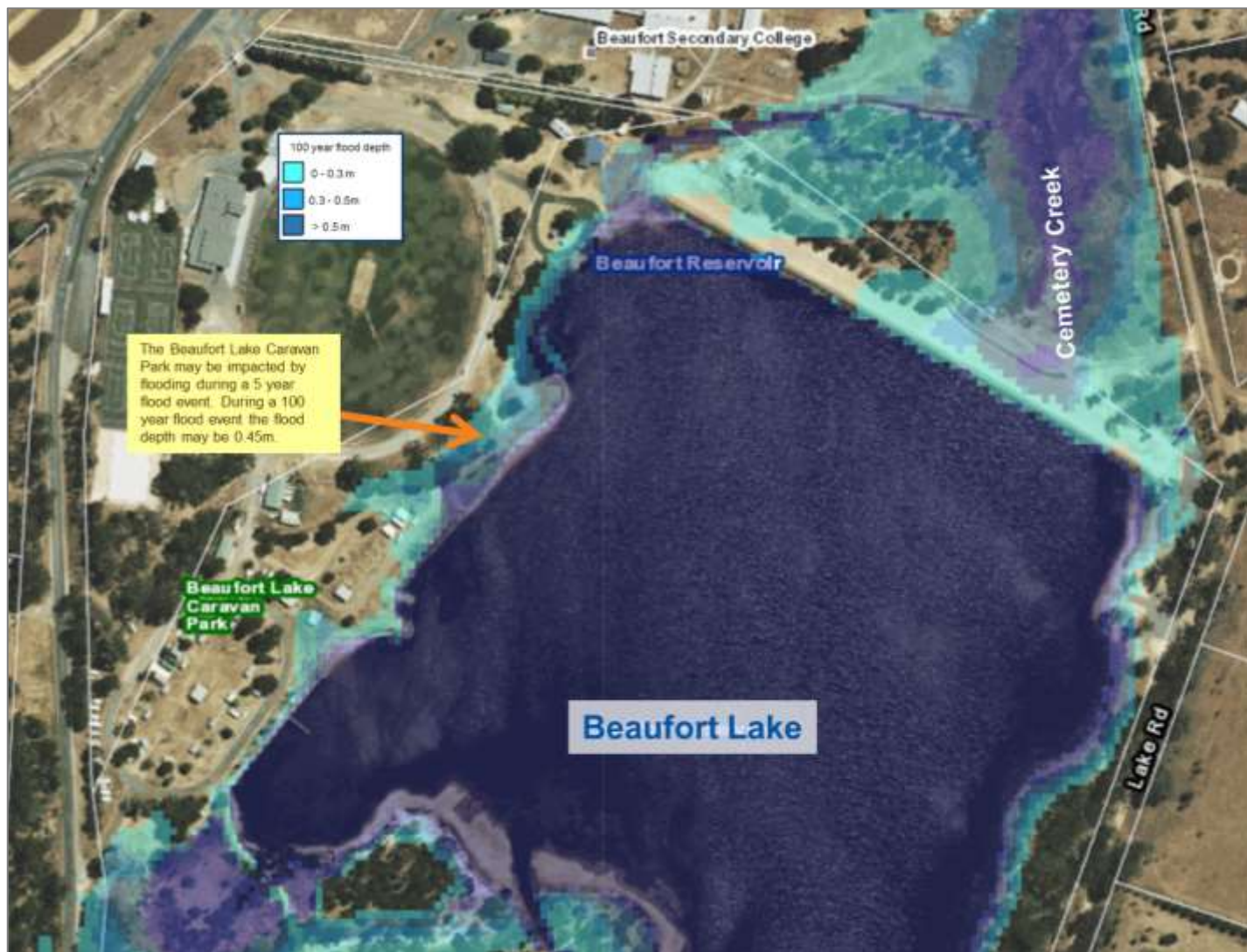
Flooding surrounding Beaufort Lake during a 100 year flood event (Water Technology 2008).
