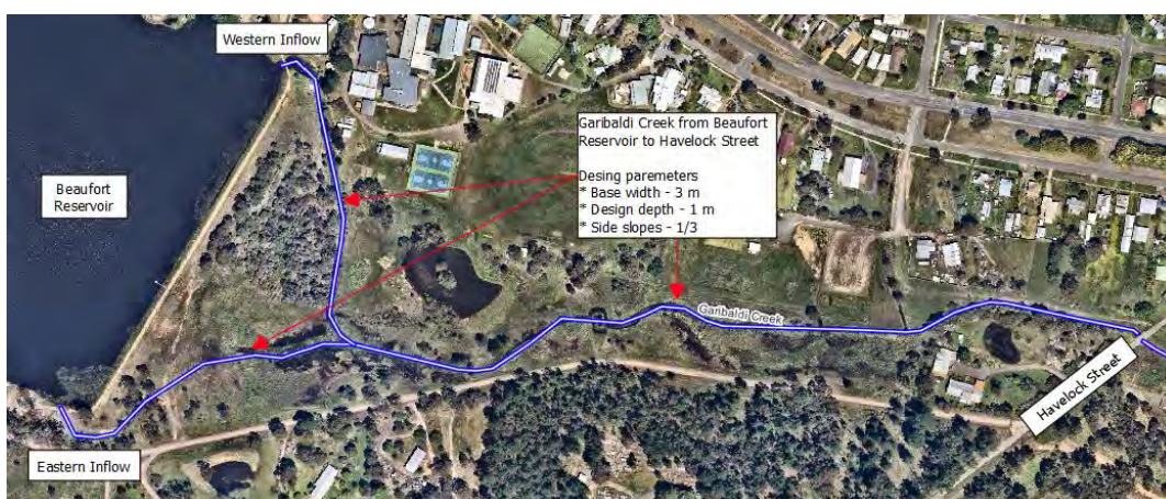
Plate 5: Design parameters from Beaufort Reservoir down to Havelock Street
