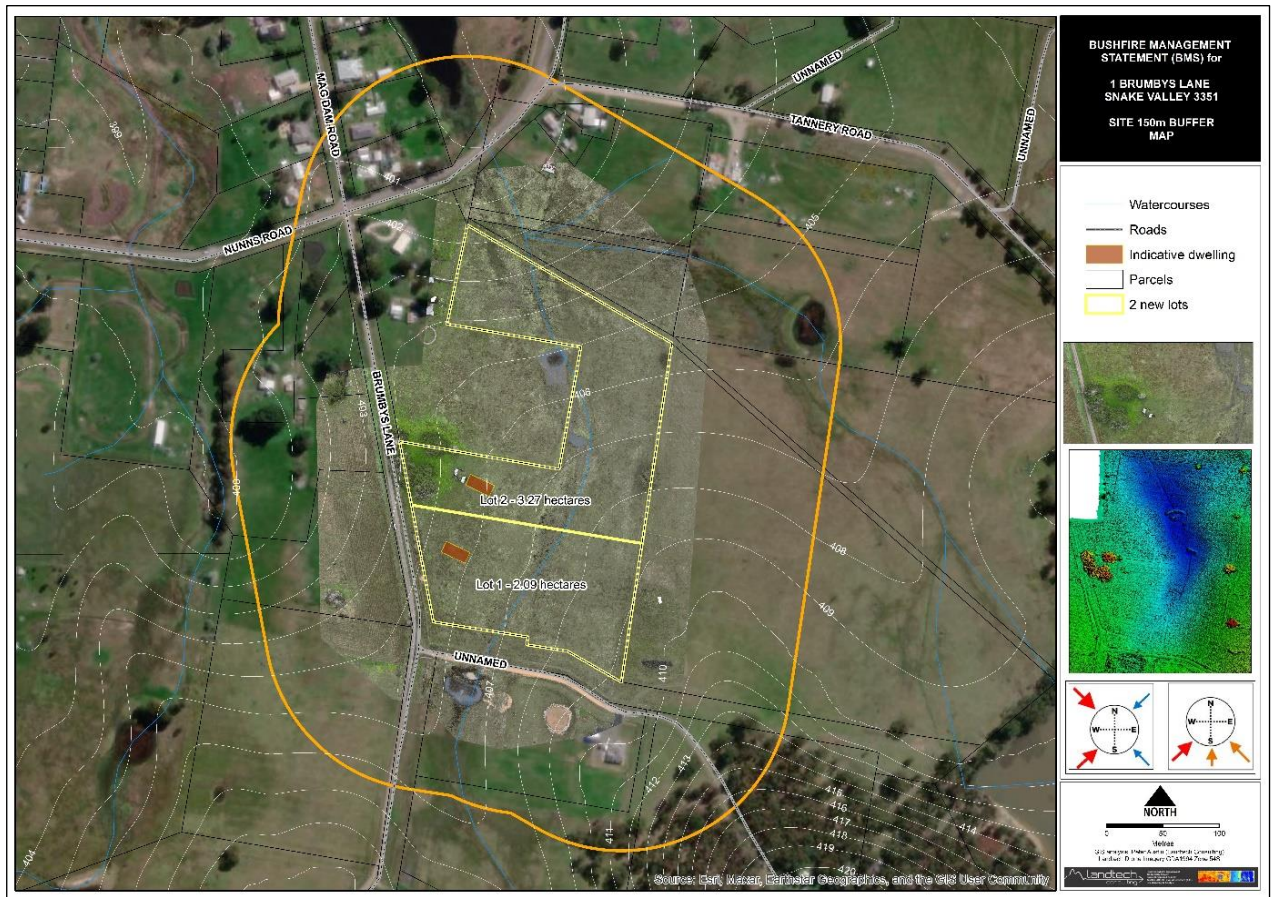
Figure 13 - 150m site buffer map and potential bushfire risk sources within and beyond the site.
