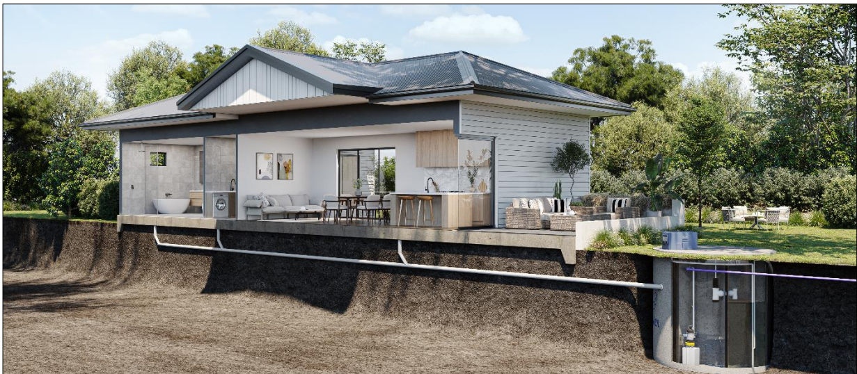
Figure 32 – In-situ view of house connection to treatment system (Source: Taylex 2023).
