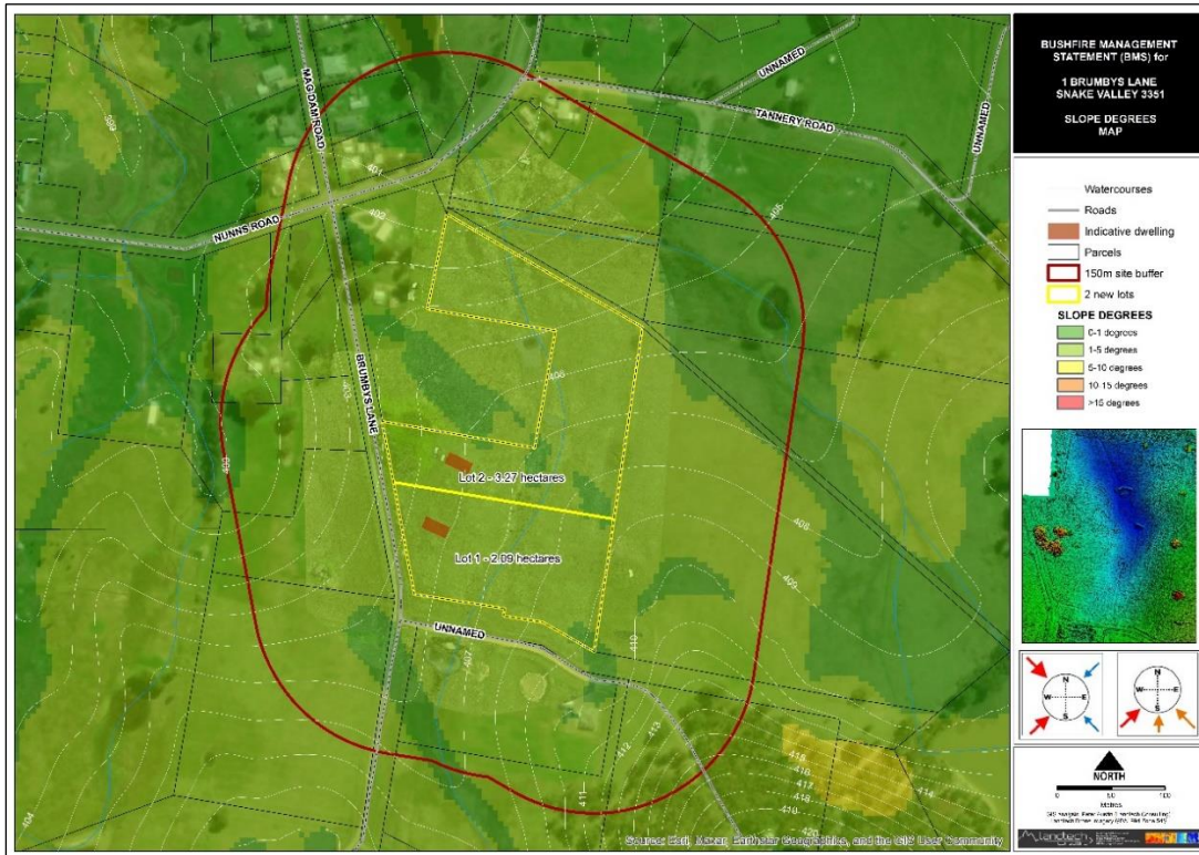
Figure 22 - Slope map (in degrees fall) showing the flat to lightly-sloping nature of the subject site.
